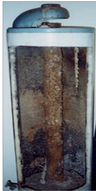
Fig. 6. Severely corroded water heater. Photograph from WaterHeaterRescue.com.
