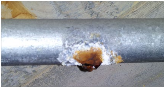
Fig. 3. Corrosion from a Pinhole Leak in Galvanized Steel Piping Photo courtesy Levco Builders.
