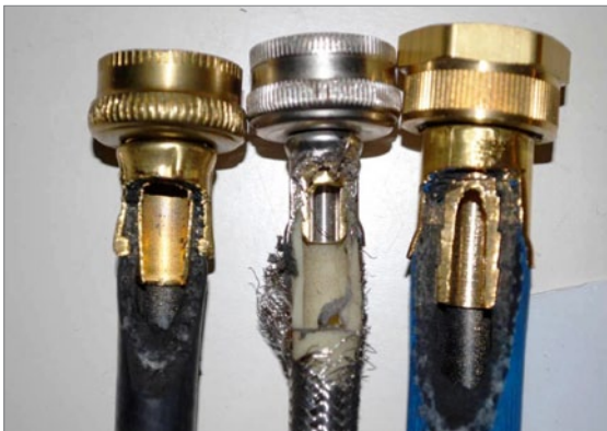
Fig. 5. Left to right: Cross sections of a standard black rubber hose, a plastic hose with braided stainless steel covering, and the Floodchek hose. Photo by SCM Engineering.
